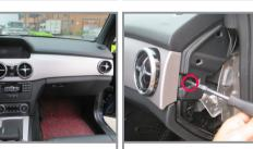
64. Connect the connector 65. Install the original fan 66. Fix the screws of emergency lamp
