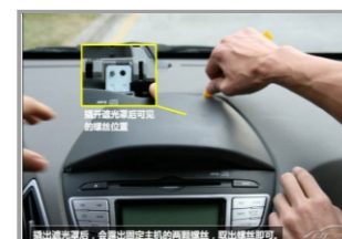
4. After prying-out the original frame, you will see 2 screws Remove them.
