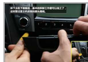
5. Pry-out the original bottom frame
