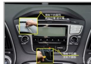
3. Pry-out the original upper frame ( see arrow)
